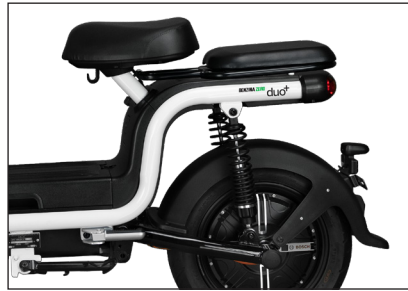
Rack Pillion Seat — Part #: FBS01001028 Pillion Seat Cushion — Part #: FBS01002008 Footpeg Rear L/H — Part #: 84B20-CK02-00000 Footpeg Rear R/H — Part #: 84B10-CK02-00000
